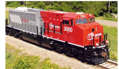
On-board fuel tender car for locomotives
