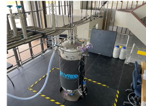
Multi-simulation LH2 testing platform
