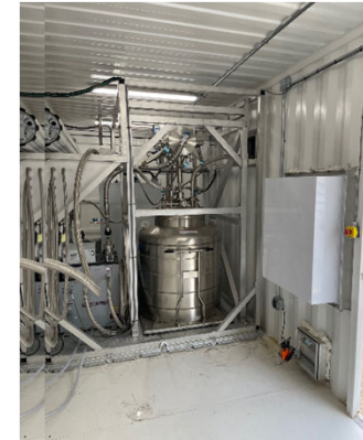
Mobile hydrogen liquefaction and dispensing
